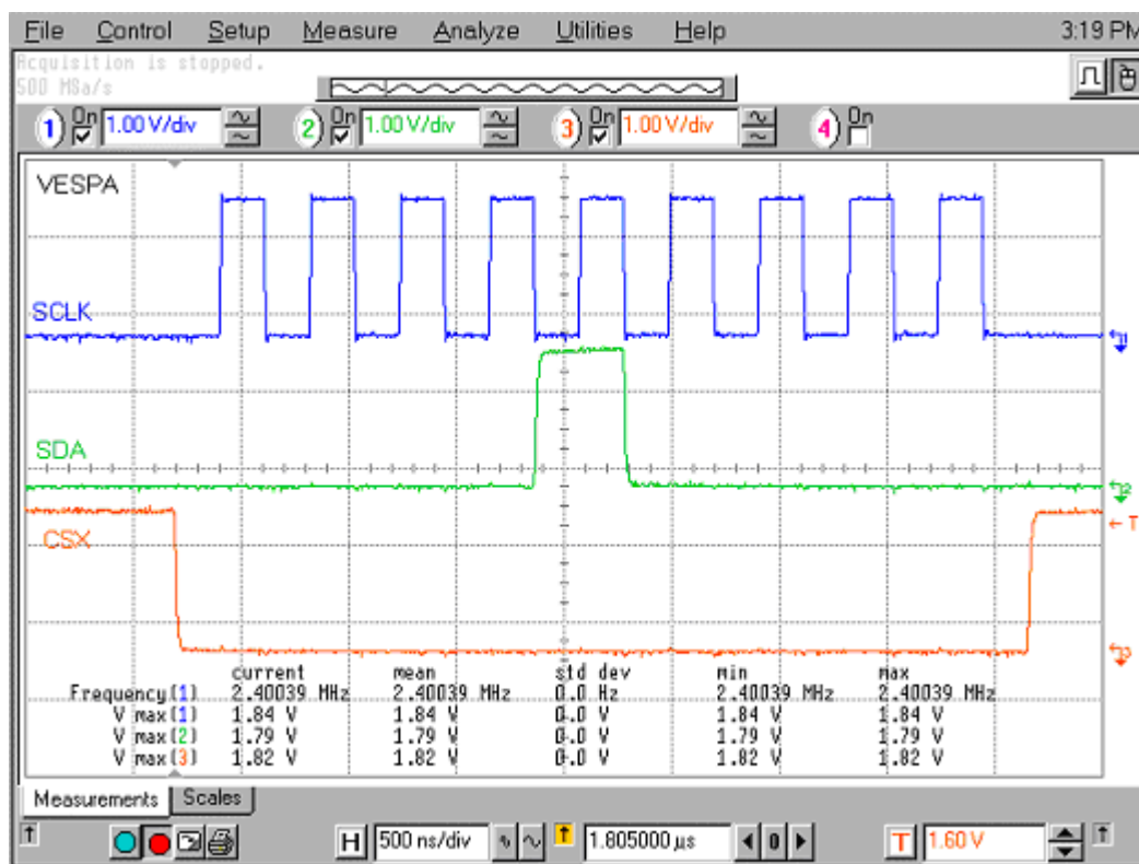
Figure 18: Waveform for the LCD Interface
