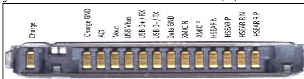
Figure 19: Tomahawk connector pin out
